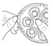
Attach so that the edges of the attachment are wrapped around the frame.
