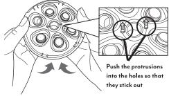
Push the protrusions in the center of the attachment into the holes in the center of the frame.
