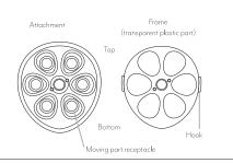
① Align the protrusions and holes in the center of the attachment, and the hooks and holes on the left and right sides. Place the frame on the attachment and push the protrusions into the holes as shown in the figure below.
